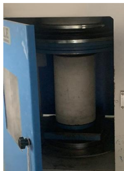
Figure 2. Experimental testing of compressive strength of concrete using RFCC
