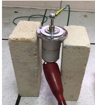
Figure 5. Vacuum contact assembly in VCB, Test Evaluation
